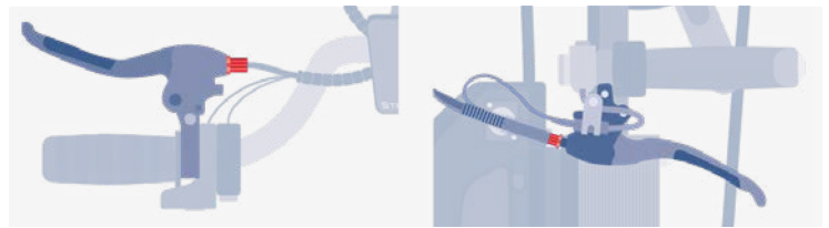
Abb. 81: Tighten the cable on the brake lever
