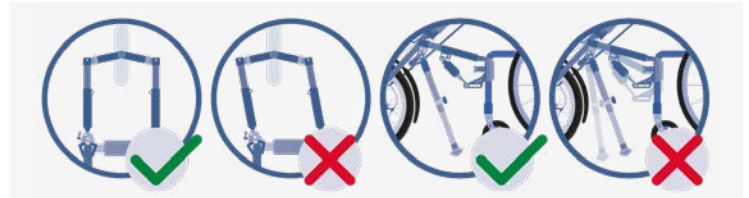
Abb. 27: Positive and negative examples of the frame position
