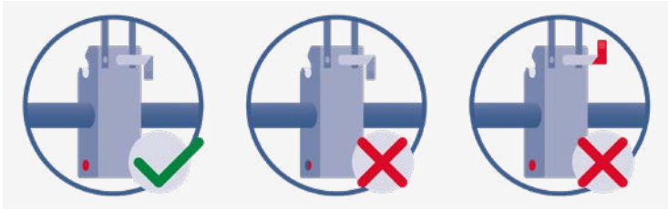
Abb. 43: Positive and negative example: bolt fully extended and locking pin engaged
